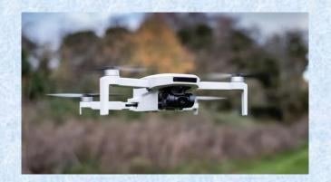
The drone is equippied with a 1/3" CMOS Sony Sensor featuring f/2.2 aperture. It can shoot 12MP photos in JPG and RAW(DNG) formats and 4K HD video at 30fps. The ShakeVanish technology helps to take more stable and smoother images within 118° FOV, a vertical +20° to -90° camera adjustment angle enable you to capture more scenes. The ShakeVanish electronic stabilization tech helps reduce the wobble from the outside, making aerial shooting more stable and smooth.
